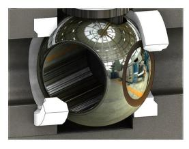
The T Seat Style designates a soft seat material. There are many seat materials available with TFM being the standard option. A metal lip on the body and tailpiece provides fire safety and meets API 607 requirements.
