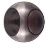
Jarecki's patented phantom port design provides a ball valve having an increased operational life and seat life by preventing the working surfaces of the ball from interfering with the valve seats due to deposits of scale, corrosive pitting or build up of film from the surface fluid. This allows free turning over a longer time period and reduces costly down time.
