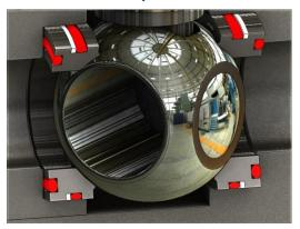
A double seal design providing both spring loading and excellent sealing capabilities. There is no area for media to build up behind the seat, which prevents the valve from locking up.
