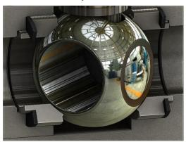
A series of Graphite seal rings behind the metal seat prevents media from building up behind the seat. The rings also allow for expansion of the internal valve components in high temperature applications. This design is great for applications involving fine solids as the graphite prevents the media from building up behind the seats.
