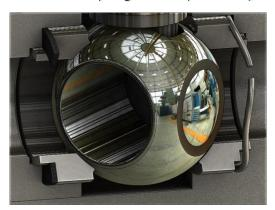
For unidirectional applications. The sealing seat is available as a separate seat ring for reparability, or integral with the tailpiece for high temperature applications. The spring seat OD seal prevents media from building up between the spring and the back of the seat.
